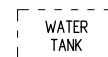
WATER TANK, REQUIRING INTERNAL FILLING UNLESS NOTED, CAPACITY AS REFERENCE, NO ENCLOSURE
