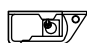
WASH HAND BASIN - POLYETHYLENE - GREY - HSE COMPLIANT SIZE & COLD TAP ONLY - WATER TANK CAPACITY 60 LITRES - REQUIRING INTERNAL FILLING UNLESS OTHERWISE SPECIFIED - WASTE DISCHARGES INTO COMPANION WC TANK WHERE FITTED
