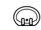
WASH HAND BASIN - VITREOUS CHINA - COMPACT SIZE - HOT & COLD BASIN PILLAR TAPS
