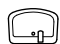
WASH HAND BASIN - VITREOUS CHINA - HSE COMPLIANT SIZE - COLD BASIN PILLAR TAP ONLY
