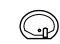
WASH HAND BASIN - VITREOUS CHINA - COMPACT SIZE - COLD BASIN PILLAR TAP ONLY
