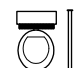
WC PAN - VITREOUS CHINA - WHITE - DISABLED LOW LEVEL, CISTERN 6 LITRES, TOILET SEAT & GRAB RAILS
